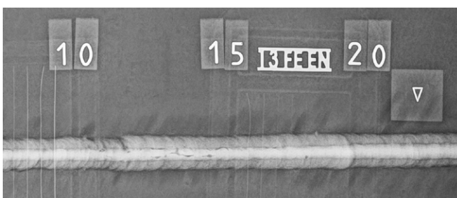
DXR Flex: FE 10mm – SWSI, X-Ray ISO 17636-2 | Class B achieved | Powered by Flash!
